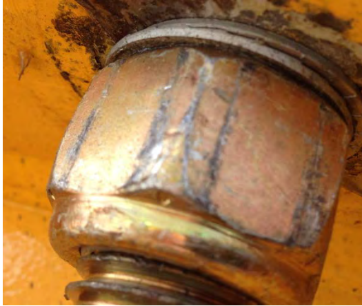
Poor lock installed
