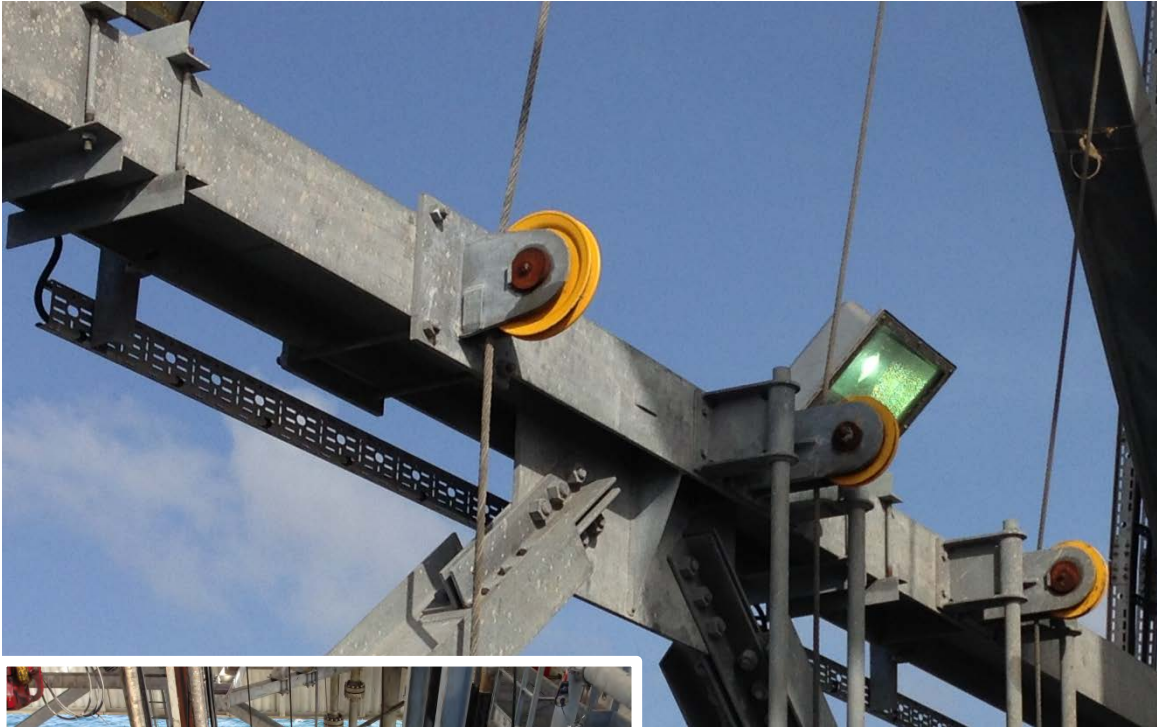
Diverter sheaves on tigger lines above the monkeyboard with no mounting frame, sheave wheel or axle retention.
