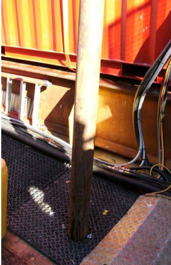
Drill pipe dropped from Drill Mast Rooster Box impaling ship's deck
