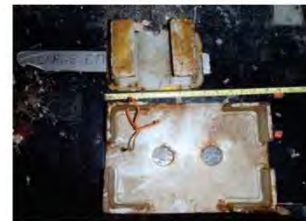
Metal pieces – Covers for trip hazards on securing point on main deck
