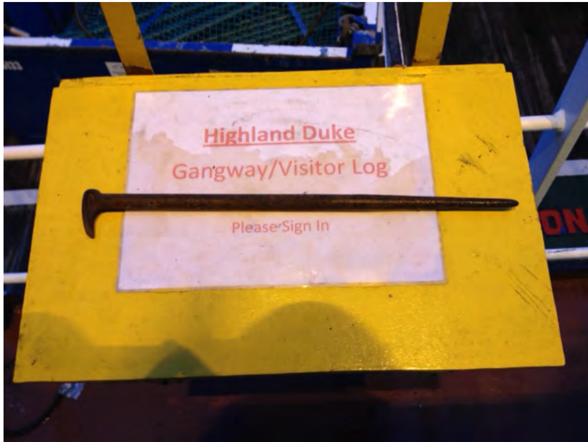
Podger bar was recovered from top of Mud Skip
