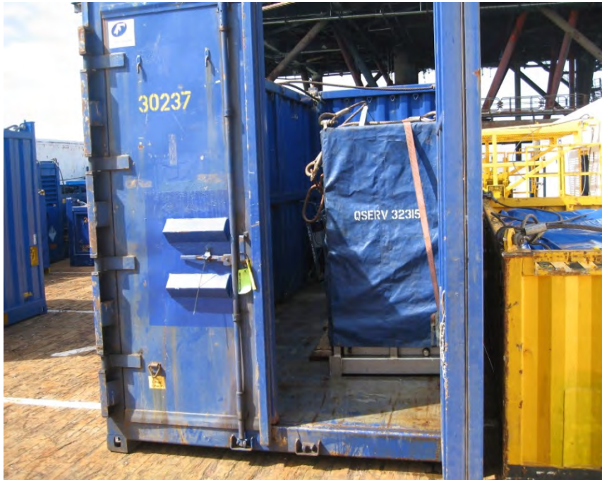
Container back loaded with doors unlocked
