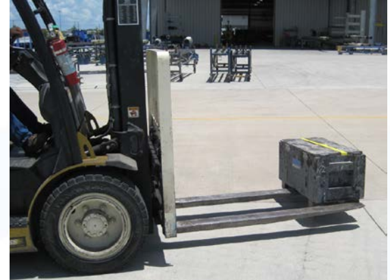
Load not all the way back and only one fork
