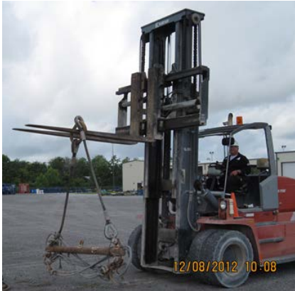
No sling directly on fork
