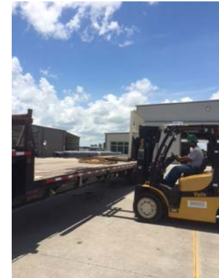
Load not all the way back and only one fork
