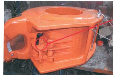
picture 6: Elevator closed, but not secured
