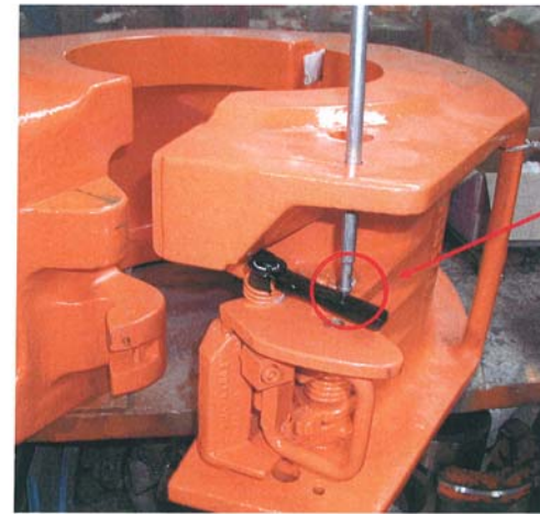
picture 8 Safety Pin can not be set, while plate is locking the hole
