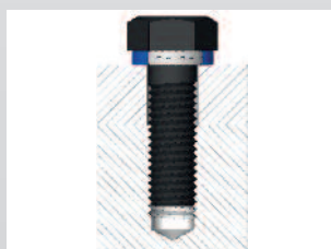
Hexagon bolt secured in a blind hole
