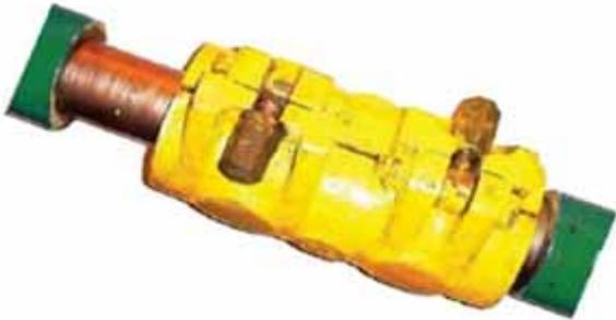
Shown (left) with bolts correctly engaged
