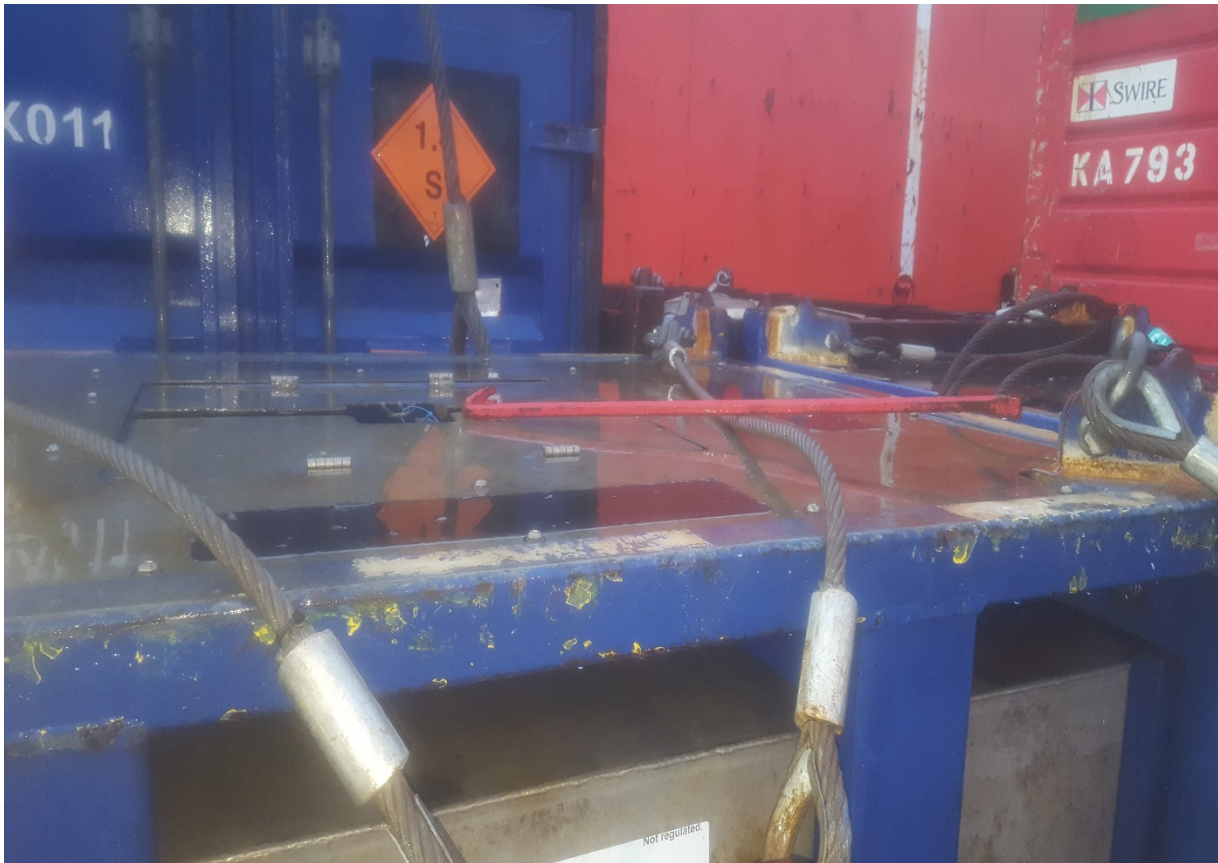
Pinch bar left on lift
