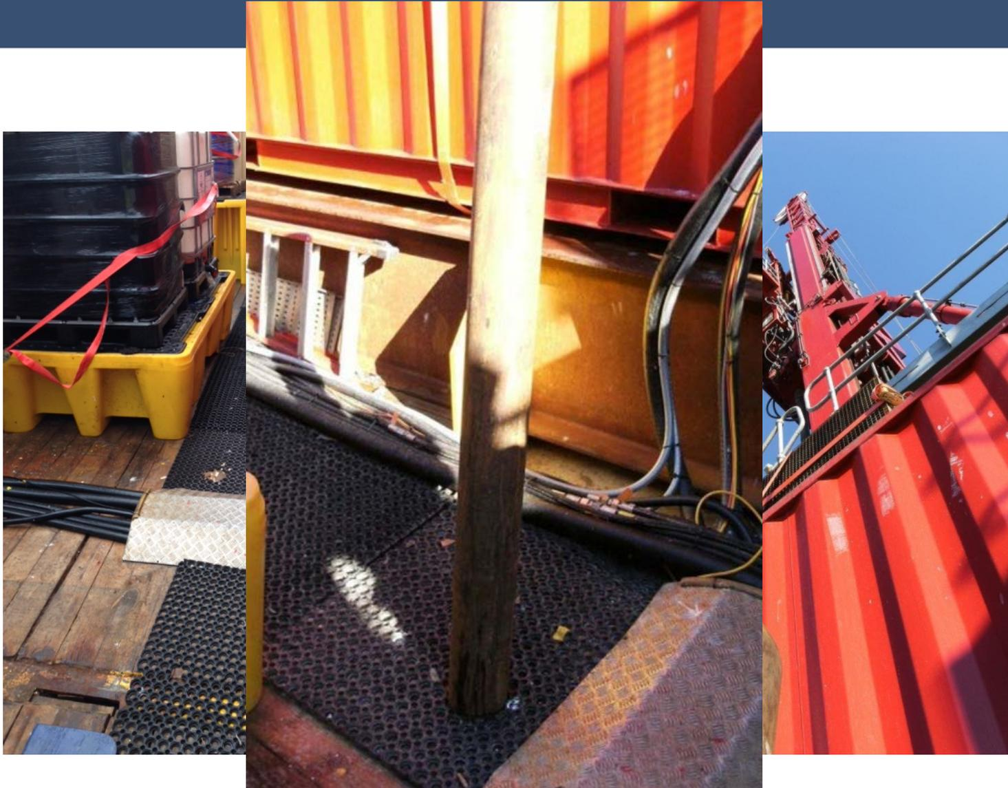
**Drill pipe dropped from Drill Mast Rooster Box**
