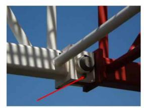
Check the pins in all boom joints have safety pin inserted and the pin is correctly secured.
