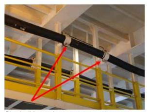
Check all hose clamps on cement hoses below cantilever are properly fitted.
