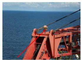
Check the warning light at the end of each boom tip. Make sure retention wire is correctly fitted and in good condition.
