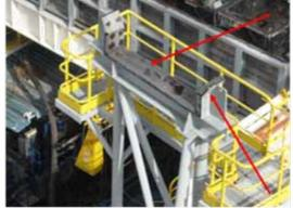
Check the wood protector on top of each boom rest is in good condition. Also check that all nuts are tight.
