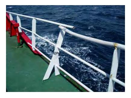
The crane was lifting a heavy lift - 12.7 tonnes from our deck, on the way up he bumped into our outer rail, on port aft, so it broke. The ship was pitching/heaving due to some swell, but within working limits, The crane operator had miscalculated the distance of the lift & and movement of the ship.
