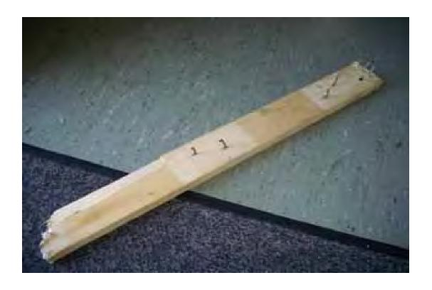
Crane operator noticed what looked to be a loose section of packing case wood on top of the crate. Once outside the 500m zone inspection showed it to be a section of packing case timber approx. 25mm x 75mm x 700mm long with six exposed nail ends some 40mm long.
