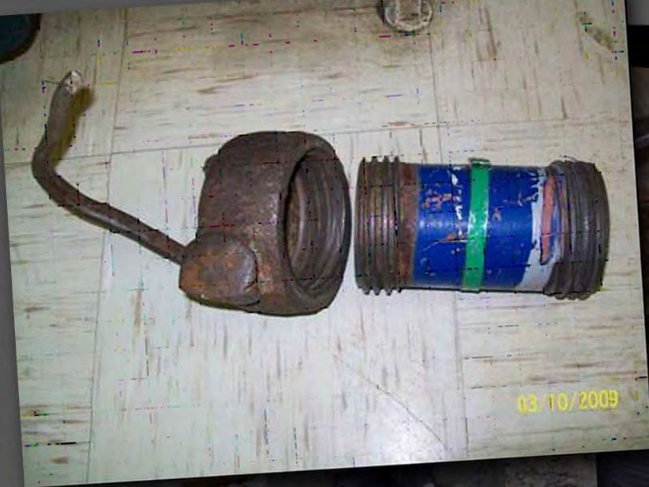
Rig fabricated, non-certified lifting device
