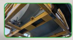
stainless steel forklift pockets Prevents rust and therefor loosening rust plates (dropped objects)
