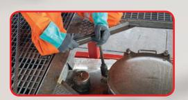
manhole cover requiring tools Expensive (EX) tools required, risk of damage to gaskets and leakages due to much force
