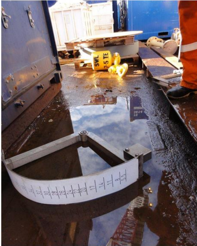
Final position of inclinometer on pipe deck
