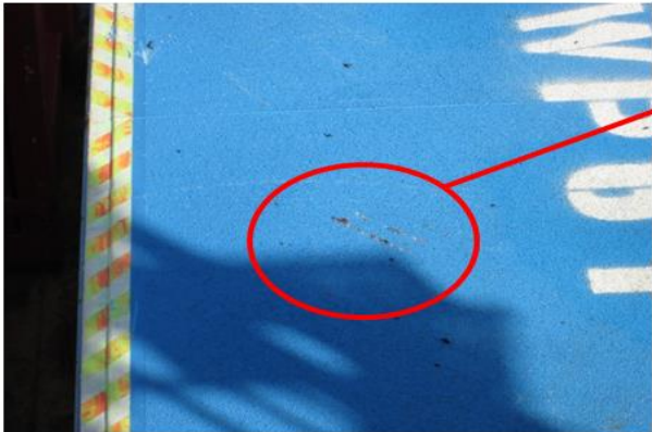
Initial impact point on top of Optima workshop container (starboard aft main deck)
