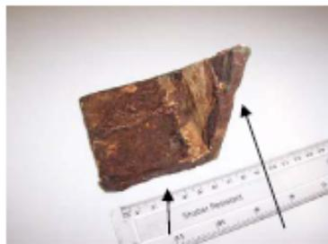
Original full weld contact corroded away
