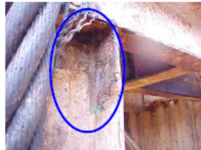
The dropped bracket came from the TDS blower frame (part of an old frame replaced some time ago). During previous derrick inspections the bracket appeared to be fully welded on to the derrick structure.
