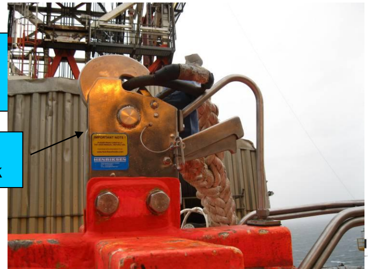
The Henriksen hook with the damaged trigger handle
