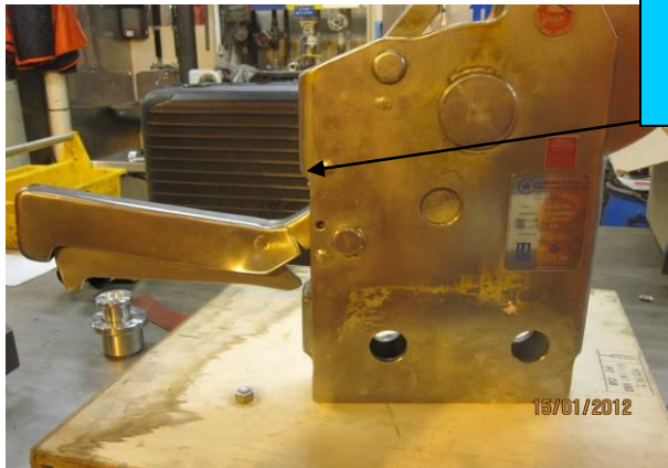
The Henriksen hook with the damaged trigger handle
