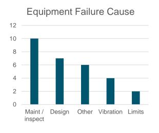
**Equipment Failures** were primarily attributed to inadequate maintenance or inspection regimes.
