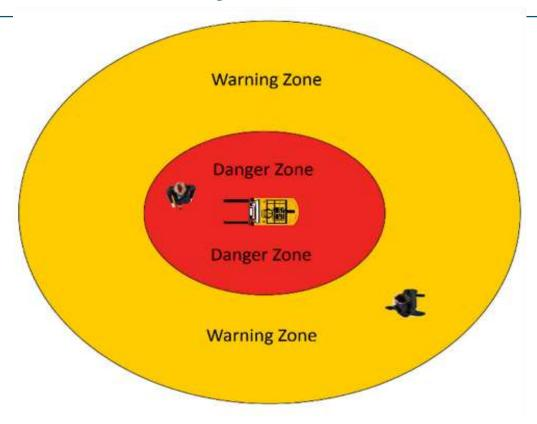
10 feet Danger Boundary from forklift 20 feet Warning Boundary from forklift
