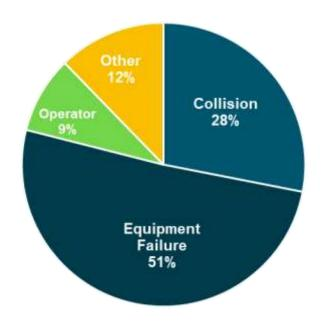
**Equipment Failure** and **Collisions** were the two main causes of dropped objects, accounting for over <sup>3</sup>/<sub>4</sub> of all events.
